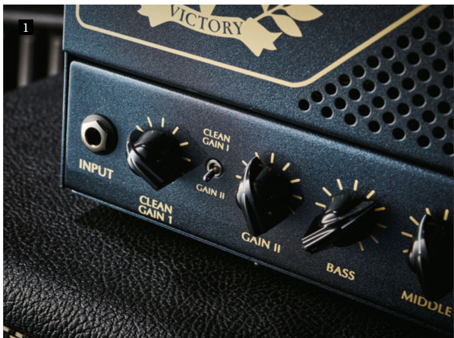
1. The front control panel is straightforward and easy to navigate, with a classy look thanks to the new paint job. There's a new Presence control, and a Clean mode for Gain I, accessed from the front-panel toggle switch or a remote footswitch
